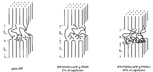
Figure 12 Schematic models of the lamellar structure of iPP phase crystallized under controlled undercooling from melts of plain iPP and iPP/aPMMA/uPP-g-PMMA blends.
